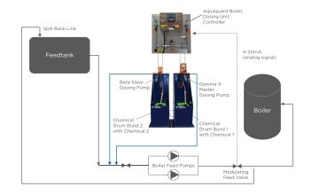
A typical installation shows the signal from the boiler feed pumps linked to the Aquaguard BW controller and proportionately driving the chemical dosing pumps. Boiler treatment chemicals are dosed into the feedwater suction line for good dispersion. Please refer to the Aquaguard BW manual for more detailed drawings and installation instructions.
