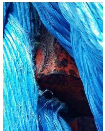
Picture 2 – A sharp edge, cutting fiber in the mooring rope
