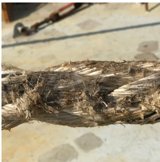
Surface abrasion on conventional ropes
