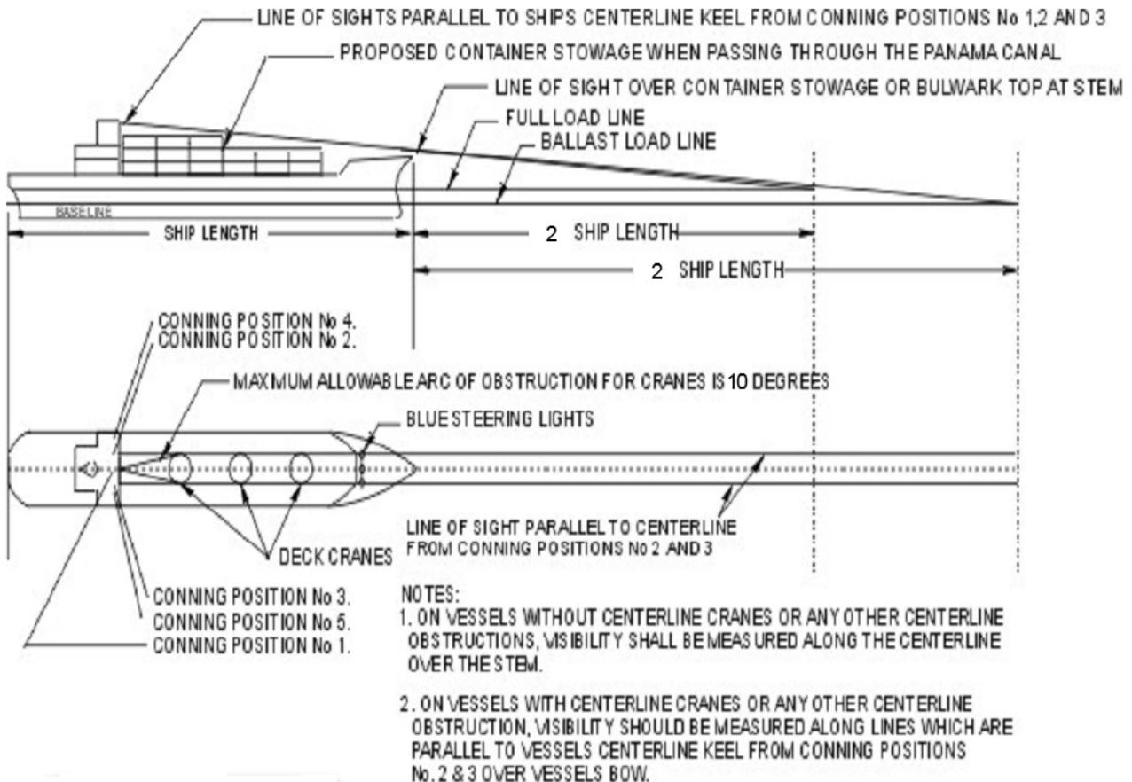
**FIGURE 4 - Normal Conning Positions**
