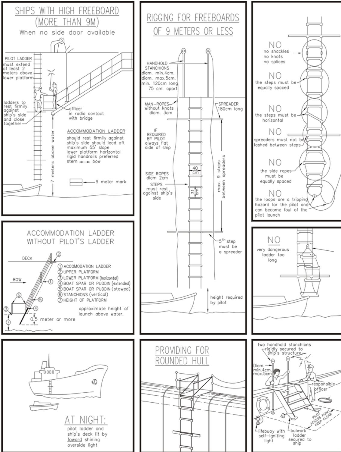
FIGURE 8 – Panama Canal Required Boarding Arrangements
