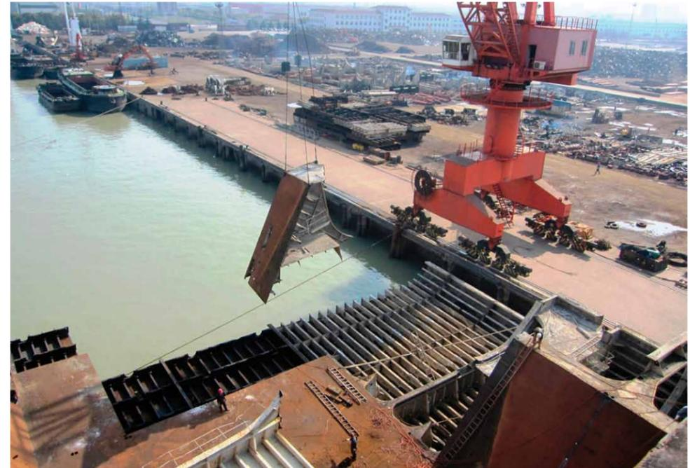
During 2013, three group vessels were recycled of which we owned two – MV Tampa and MV Terrier. Our vessels were recycled at green recycling yards in China.
