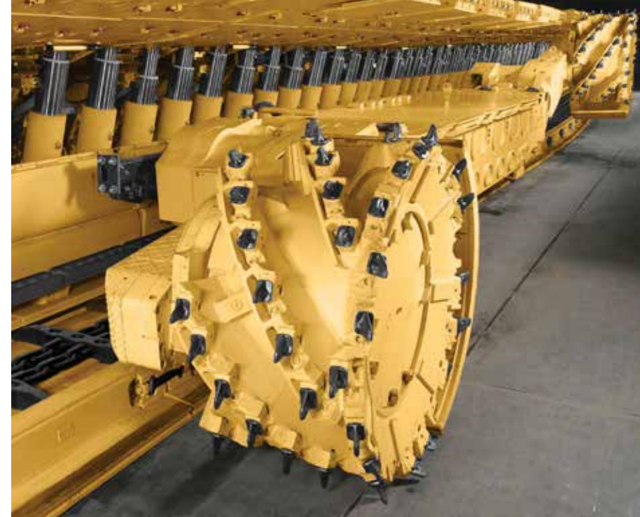
A longwall shearer is used to cut coal from the coalface, the part of an underground mine where the coal is cut out of the rock.
