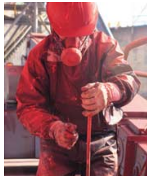
A fouled hull and propeller can increase vessel resistance in the water by 5-20%. During a docking, barnacles and other marine organisms are removed from the underwater hull and a new coat of tin-free antifouling applied.
